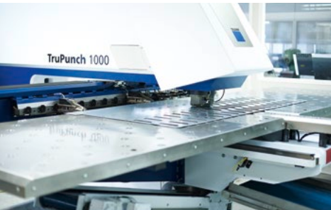
CNC sheet metal shaping centre
